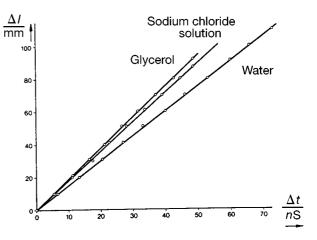
Fig. 3: Change in sound path  $\Delta I$  as a function of the change in delay time  $\Delta t$ , for water, glycerol and sodium chloride solution (temperature  $\vartheta = 25 \,^{\circ}$ C).
