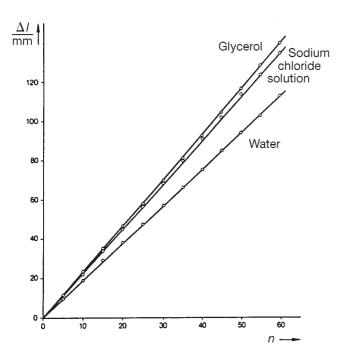
Fig. 2: Detector displacement  $\Delta l$  as a function of the number *n* of wavelengths covered, for water, glycerol and sodium chloride solution (temperature  $\vartheta = 25 \,^{\circ}$ C).
