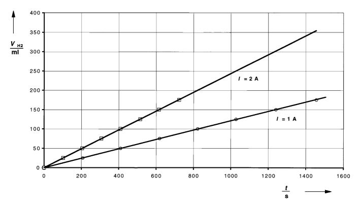
Fig. 11. Volume of the hydrogen generated by the PEM electrolyser as a function of time at different current *I*.
