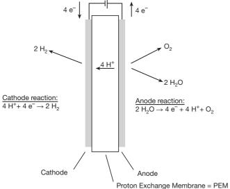
4 e 4 e O<sub>2</sub> (Air) 2 H 4 H<sup>+</sup> 2 H<sub>2</sub>O Anode reaction: Cathode reaction:  $2 H_2 O \rightarrow 4 e^- + 4 H^+ + O_2$  $4 \text{H}^+ + 4 \text{e}^- \rightarrow 2 \text{H}_2$ Anode Cathode Proton Exchange Membrane = PEM
